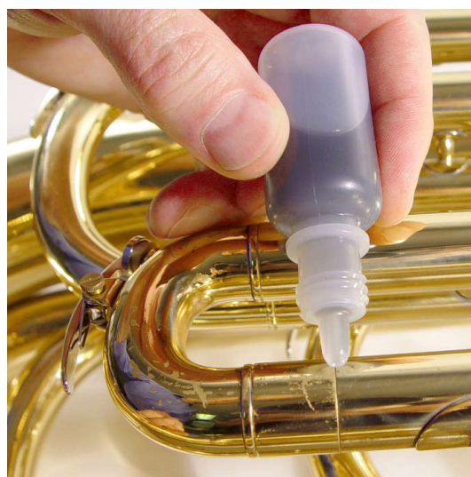
Applying penetrating oil.
