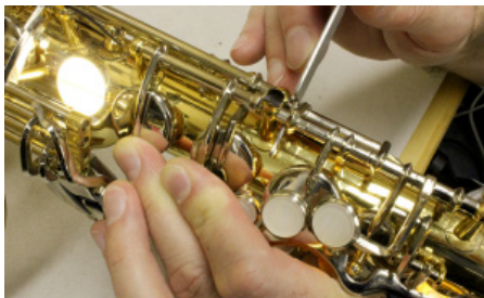
Holding A-Key and flexing foot from C back bar, with step end turned up.
