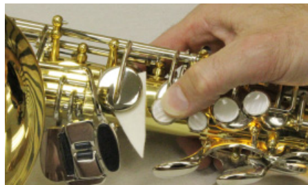
Adjusting pearl arm down and pad cup up.
