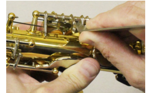
Reducing angle of C-Key arm.
