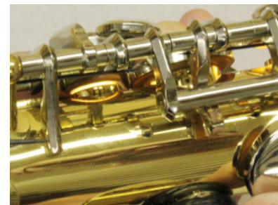
Under-adjusted LH B.
