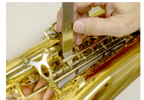
Lifting back bar of F#.
