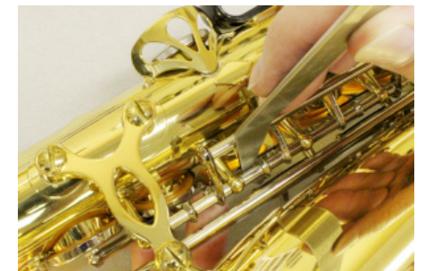
Adjusting back bar down.
