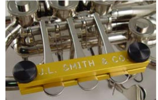
2. Loosen the rotor stop and the lever string screws and remove the old string. Don't loosen the screws more than enough to remove the old string (we don't want to lose them).
